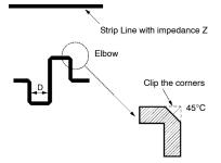
When the lines must curve, an elbow can be used as shown in the diagram. A distance (D) between the lines of approximately twice the line width is sufficient.
