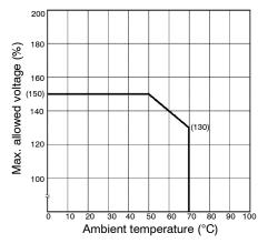
Note: The "Max. allowed voltage" is the maximum voltage that can be applied to the relay coil. It is not the maximum voltage that can be applied continuously.
